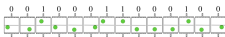
Fig. 5.10 Minimalist digital memory tape. The position of a single ideal gas atom denotes a bit. If it is in the top half of a partitioned box, the bit is one, otherwise it is zero. The side walls of the box are pistons, which can be used to set, reset, or extract energy from the stored bits. The numbers above the boxes are not a part of the tape, they just denote what bit is stored in a given position.
